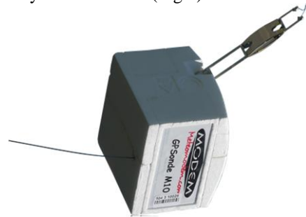
Figure 1. M10s radiosonde produced by Meteomodem including a GPS receiver, RF transmitter, temperature and humidity sensors and an auxiliary input which was used to hook up the magnetometer
